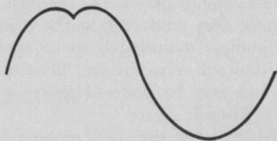
Fig. 21-10. Waveform appearance indicating nonre-entrancy.
