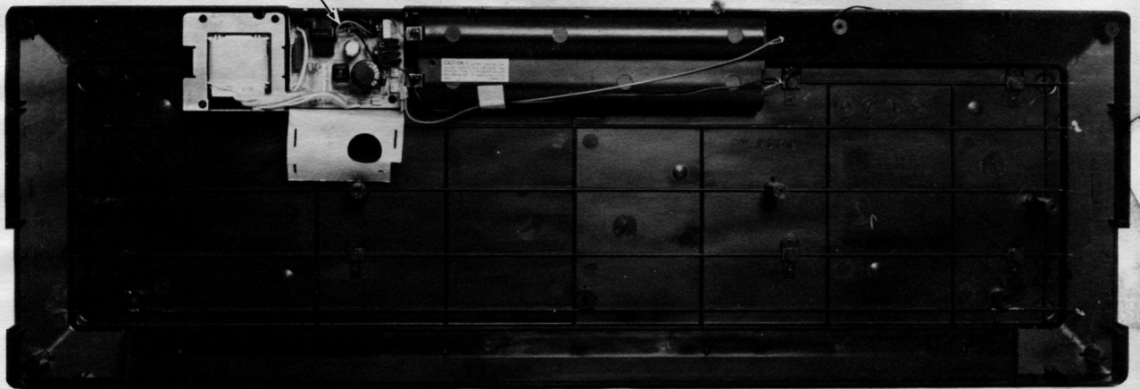
Board 8 Power Supply
